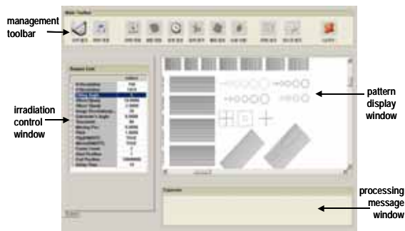
Fig. 6 Photolithographic pattern generating system
