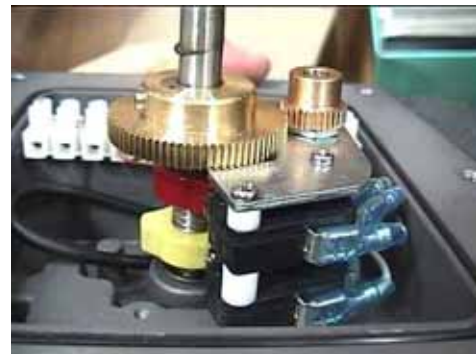
Fig. 6 Inner part of the limit switch box.
