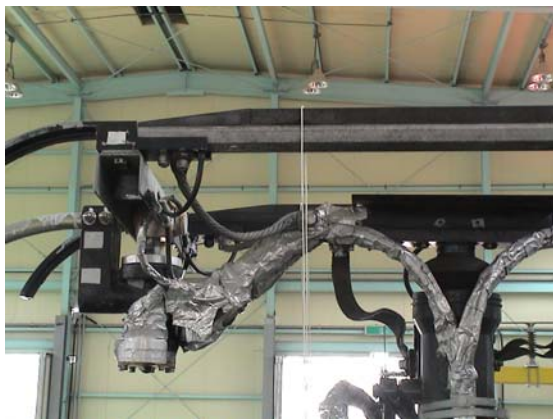
Figure 4 Connecting wire to transfer lifting force
