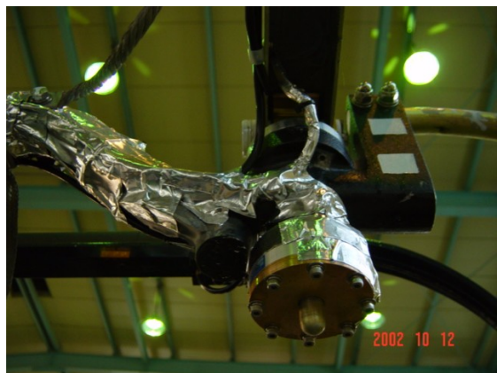
Figure 8 Load cell to measure spring force
