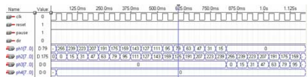
Fig. 9 Simulation result of microstep controller
