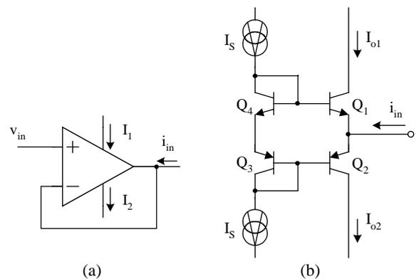
Fig. 2 Principle of the Class AB output stage
