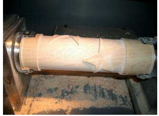
Fig. 13. A wooden roller machined by the proposed 3D machining system.
