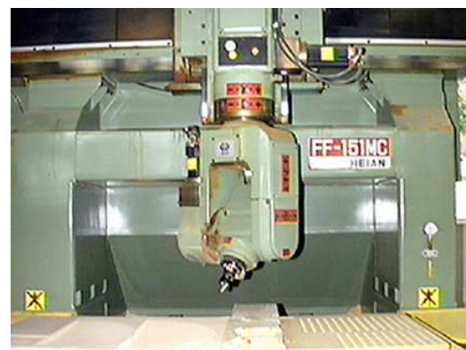
Fig. 1. 5-axis NC machine tool with a tilting head.
