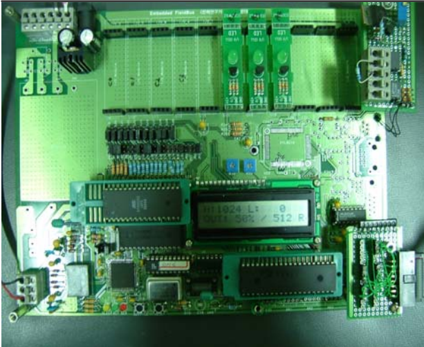
Fig.3 Developed ShortStack board
