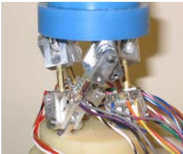
Photo. 1 Structure of the sensor
