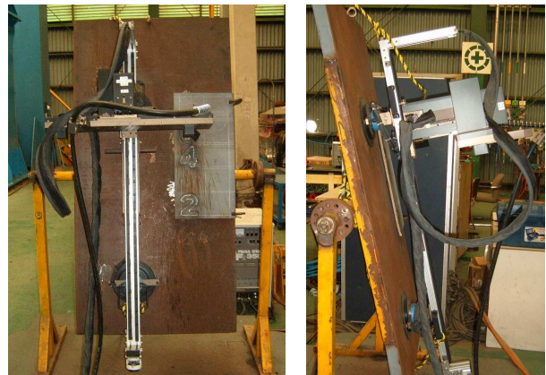
Fig. 10. Test bed for welding condition by angles
